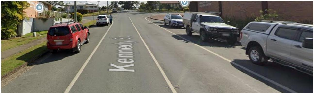
Figure 3-24: Kilcoy Murgon Road – example on-street parking with minimal clearance from traffic lanes.
