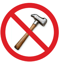
Hardened steel hammers over 2kg used on hardened steel
