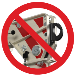
Soft slings connected directly to rhino hooks
