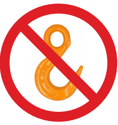
Lifting equipment and hooks without safety catches
