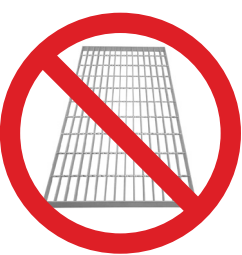
Grid mesh that is not temporarily fixed
