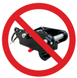
Excavator and backhoe quick hitch devices without secondary safety device
