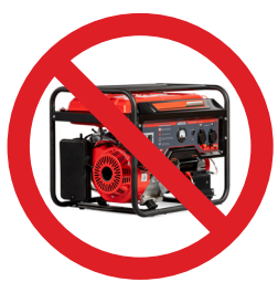
Generators not fitted with a Residual Current Device (RCD)
